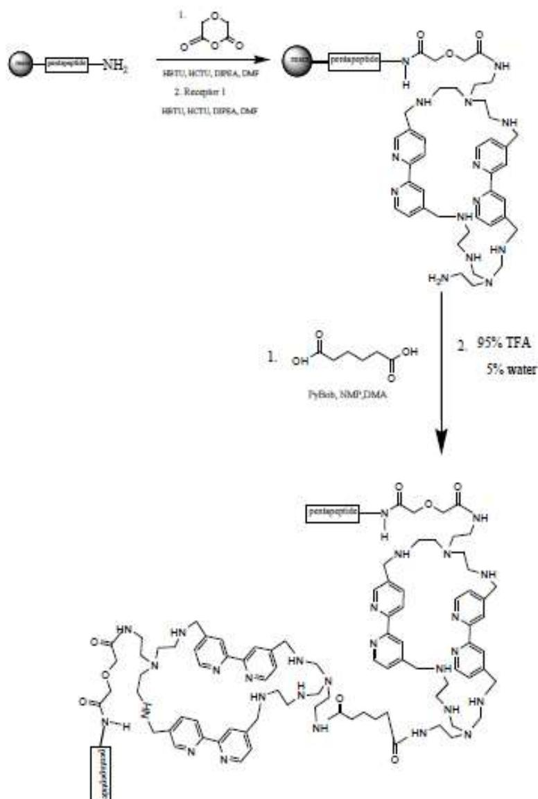
Figure 10: Linking diglycolic anhydride to Receptor 1 and the dimerization of Receptor 1 using adipic acid.
