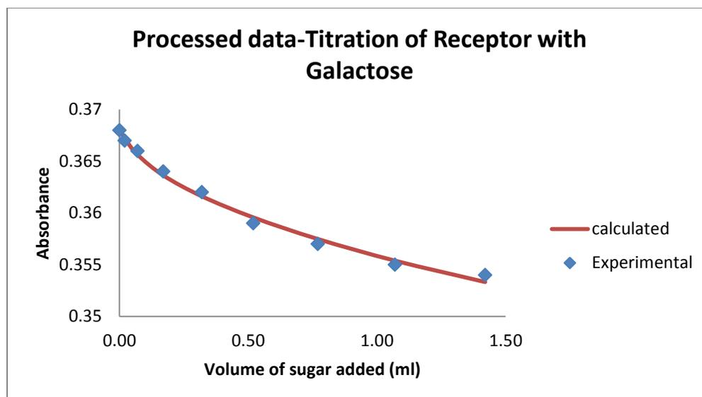
Figure 17: A plot of absorption against volume for the titration of Receptor 1 using D-Galactose (0.0278 M) @ 284.5 nm.
