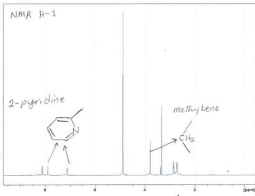
Figure 12: NMR H-1 for Receptor 1 (peaks and structure)
