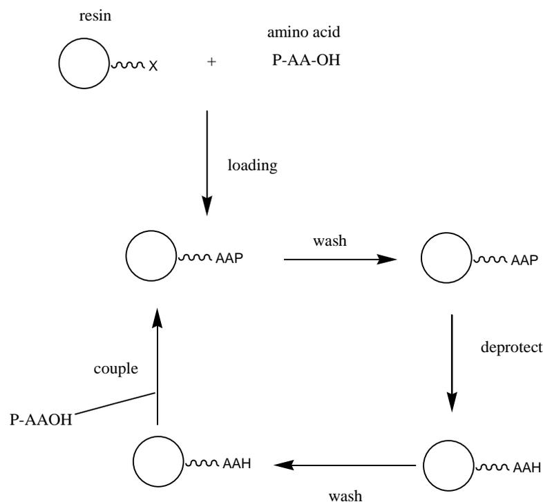
Figure 9: The general scheme for the coupling reaction
