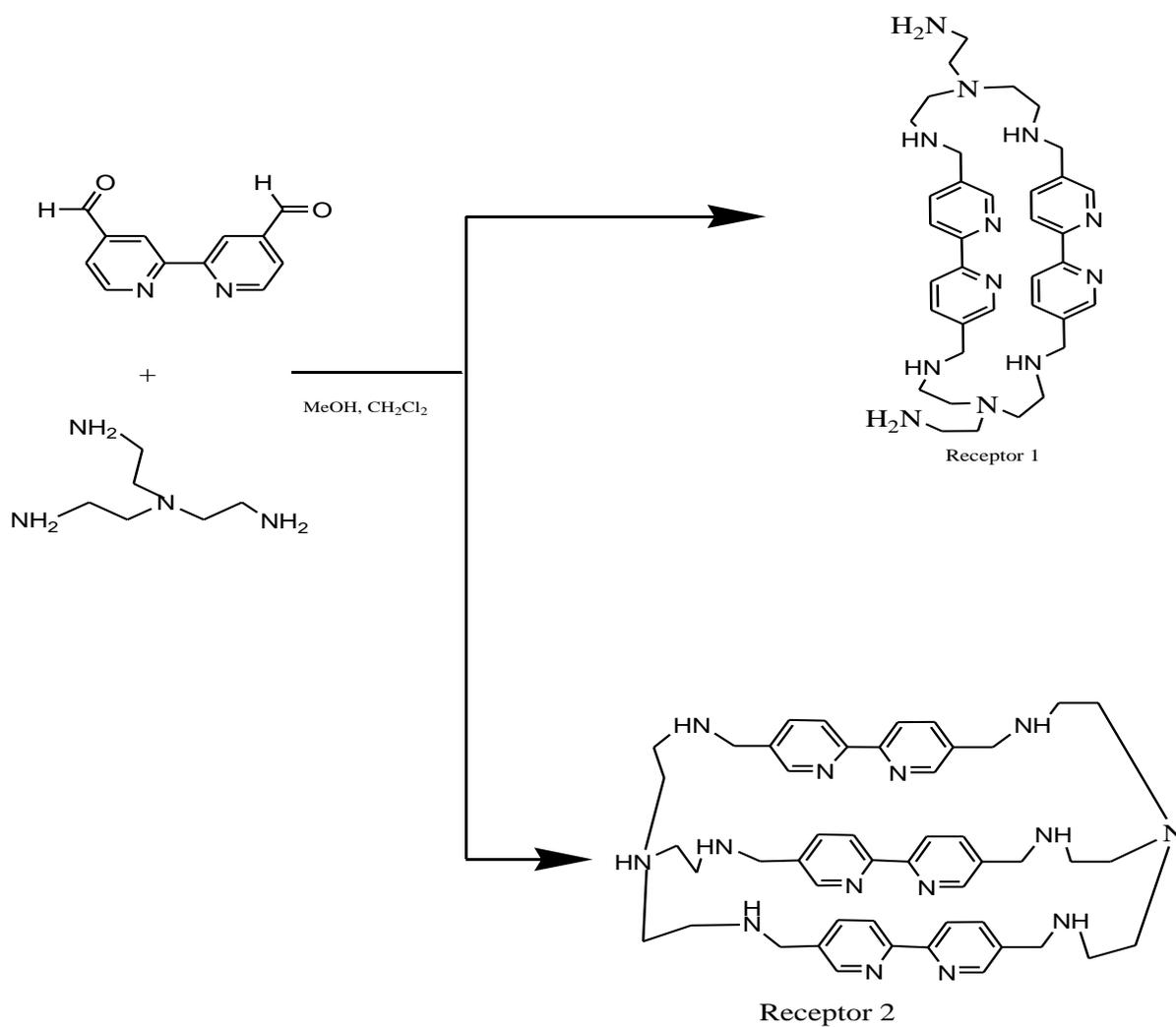
Figure 8: Synthetic scheme for production of Receptor 1 and Receptor 2
