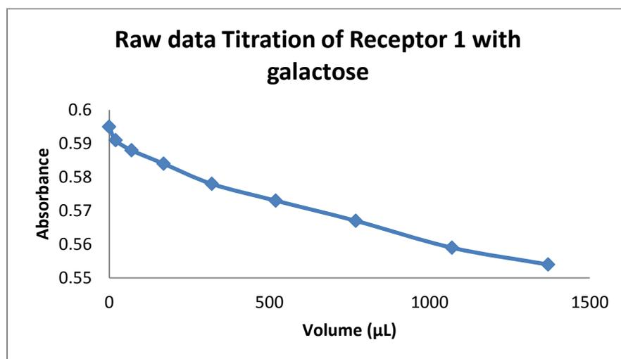
Figure 15: A plot of absorption against volume of sugar solution for the titration of Receptor 1 using D-Galactose (0.0278 molar) @ 284.5 nm.
