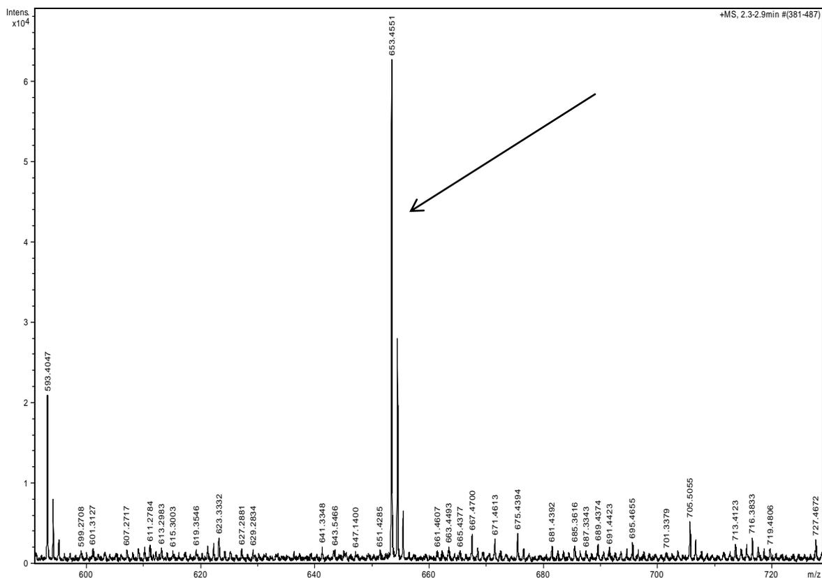
Figure 14: HR-ESI Spectrum of Receptor 1
