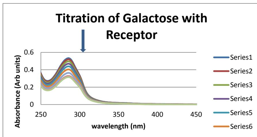
Figure 16: A plot of absorption against wavelength for the titration of Receptor 1 using D-Galactose (0.0278 molar)
