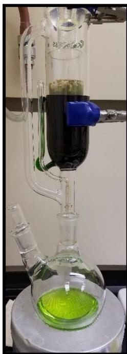
**Figure 1.** Photo of the Soxhlet extractor and setup used in this study. Ground leaves (30g) are being extracted with 210 mL of solvent.
